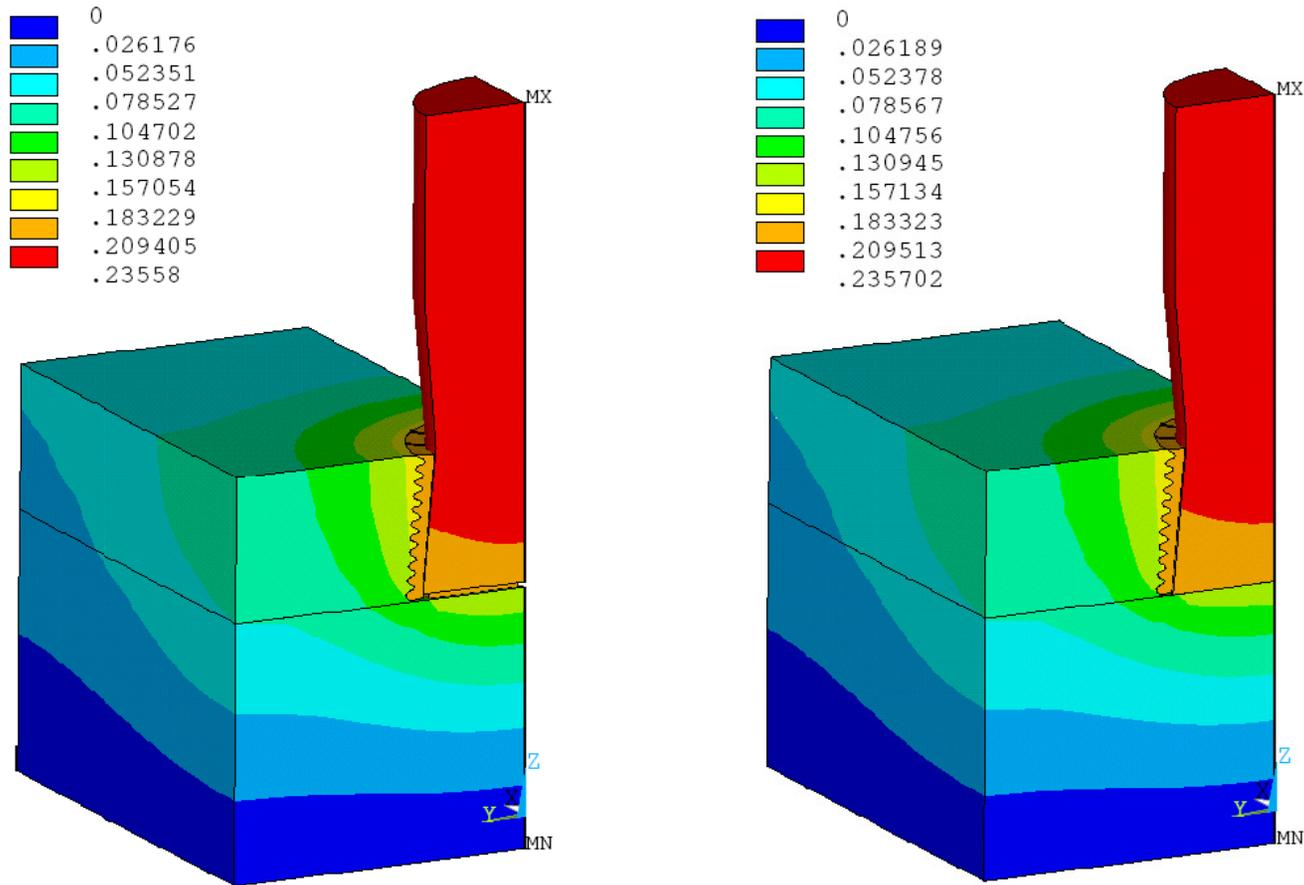
With and without cast iron under the stub
