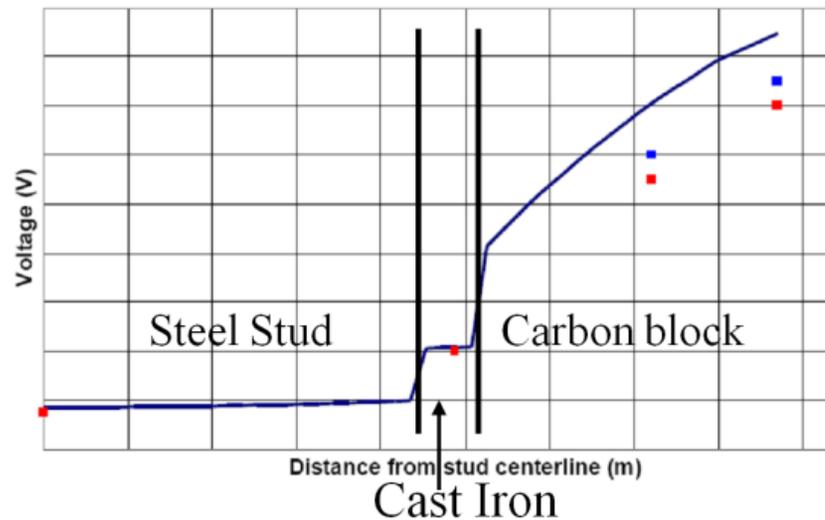
Figure 11 Anode stud voltage drop results
